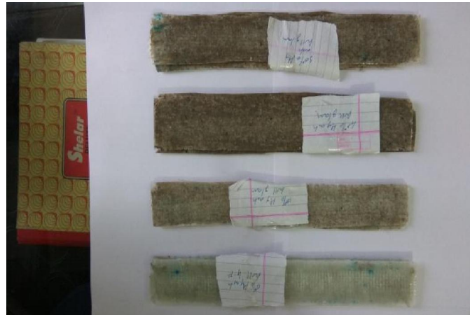
Fig.11 Test Specimens of various (10%, 30%,40%) of fly ash content and pure composite material
