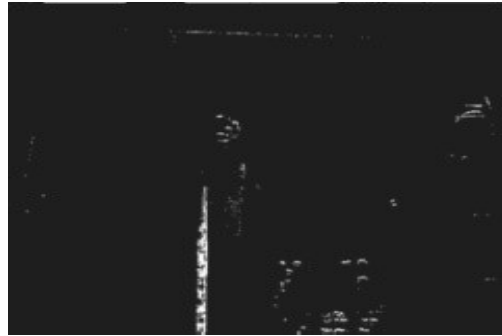
Fig 10: Binary difference between the two frames showing holes
