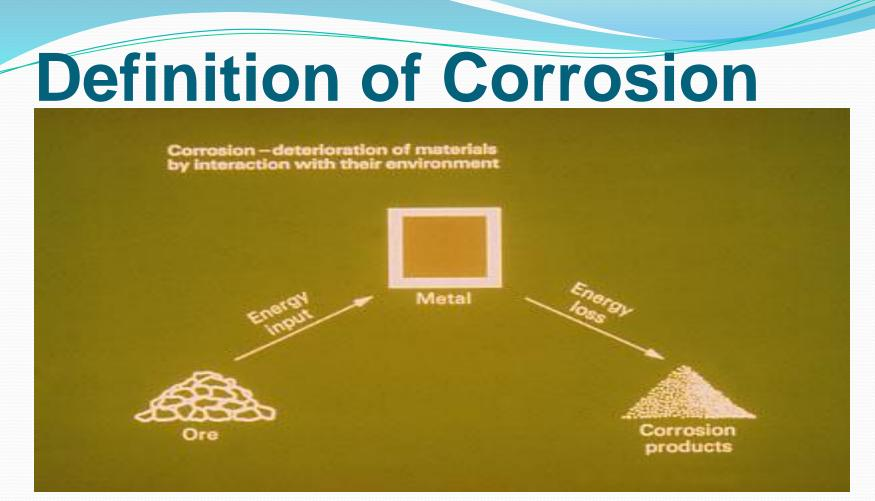
Corrosion is the deterioration of materials by chemical interaction with their environment. The term corrosion is sometimes also applied to the degradation of plastics, concrete and wood, but generally refers to metals.
