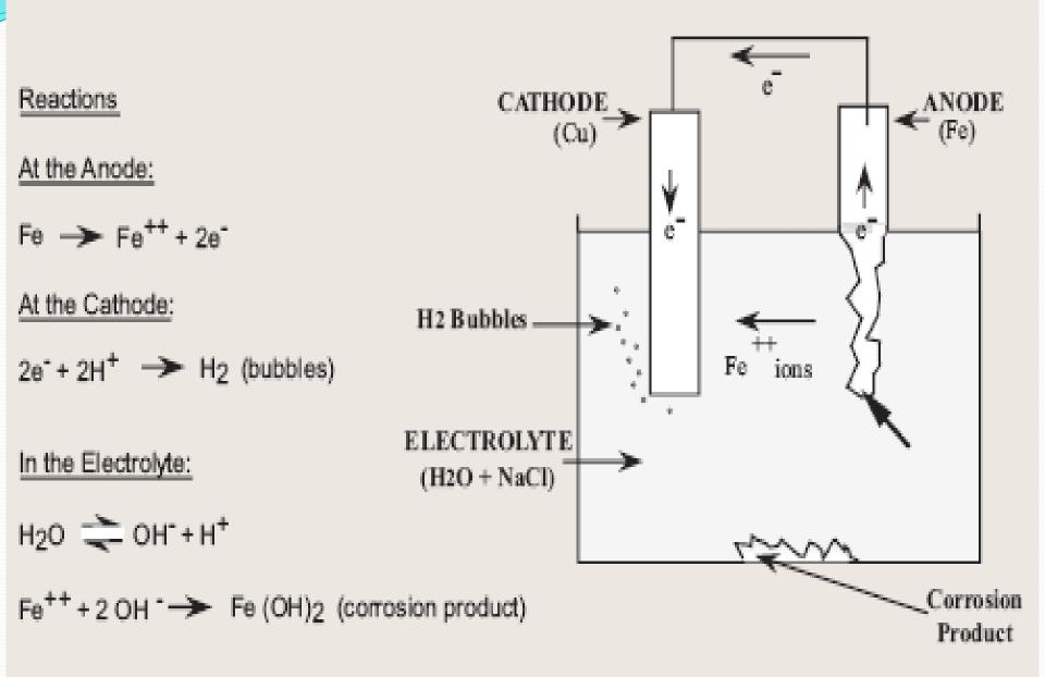
The amt of metal (iron) which is dissolved in the electrolyte is proportional to the number of electrons flowing, which in turn is dependent upon the resistance of the metal.
